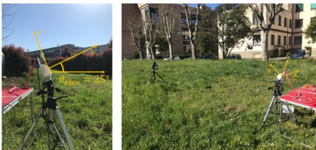
Figure 1. GB-SAR setup during the measurement in the controlled scenario.
