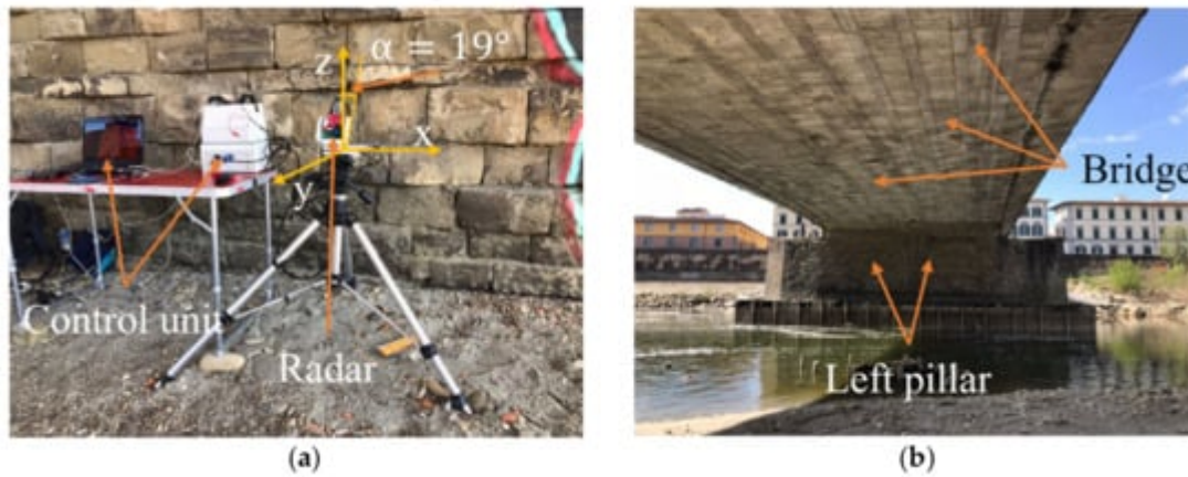
Figure 7. Radar setup (a) during the measurement campaign at Vespucci bridge (b).
