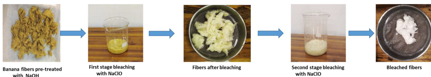
Figure 4. Two-stage bleaching process.
